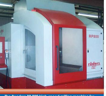
The Roeders RP 800 high-speed milling machine for hardened steel utilizes an onboard laser to direct the cutting process.
